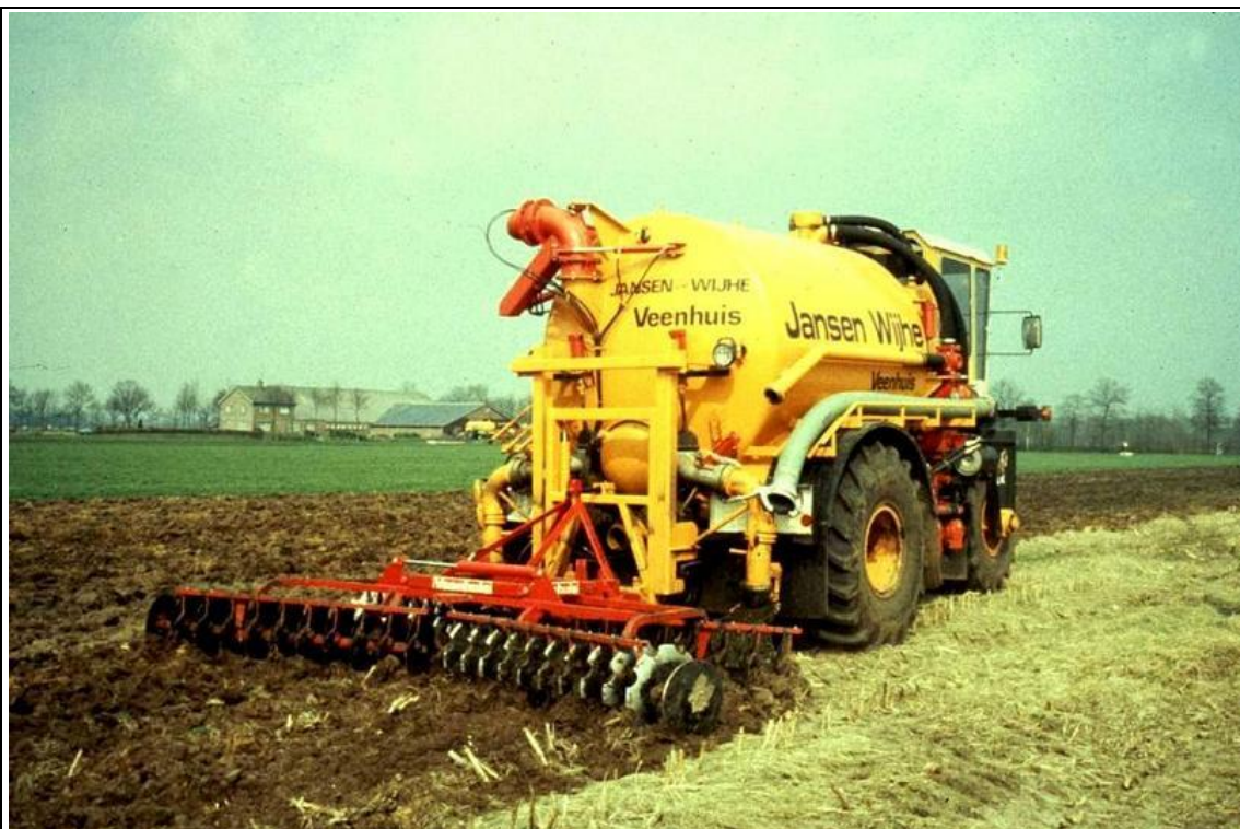
Figure 4.101: Incorporation equipment combined with a big tanker
