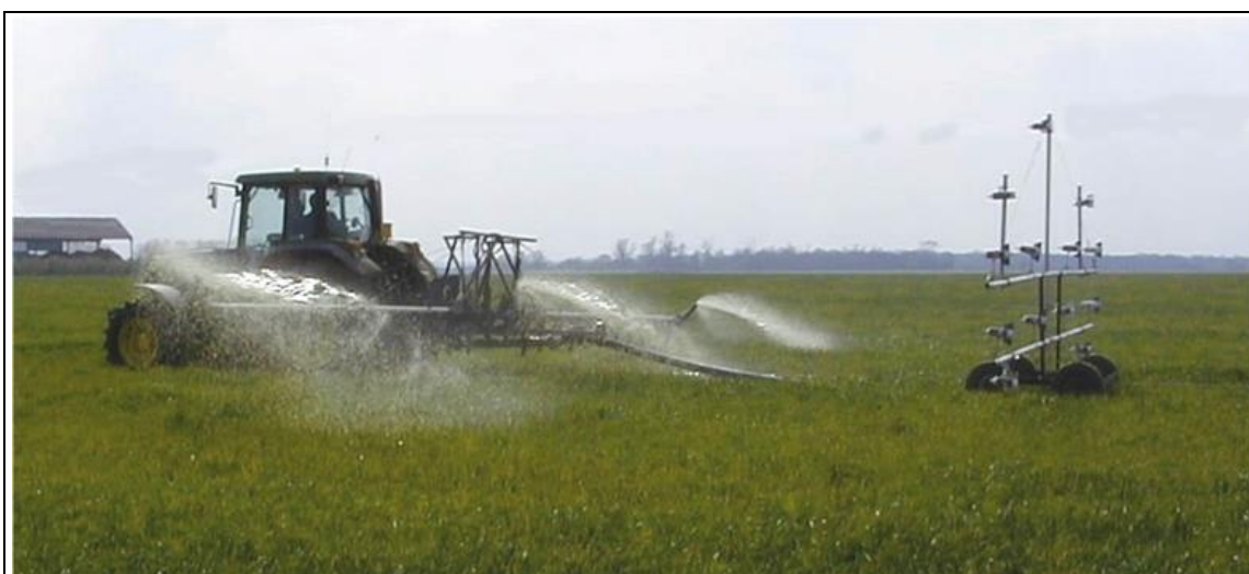
Figure 2.36: Side view of a horizontal boom with splash plate for slurry application
