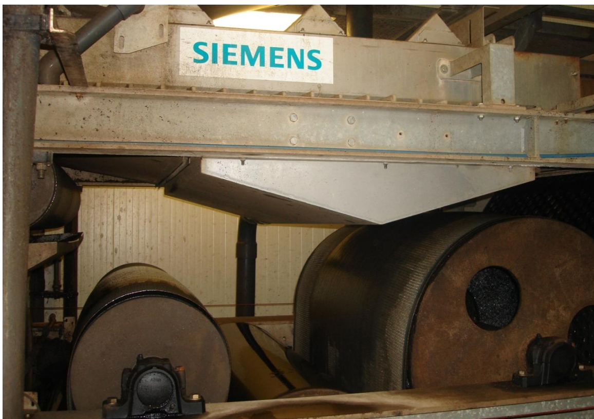
Picture C.4: Separation with filter belt press, after treatment with an additive and a polymer.
