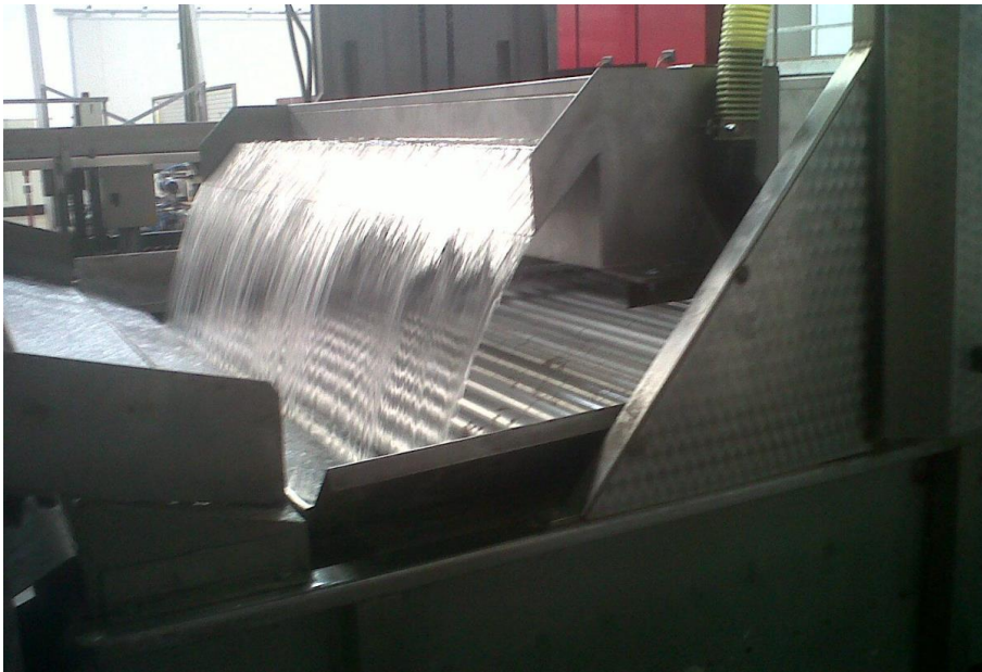
Figura 12. Balsa catarata o drencher on-line.
