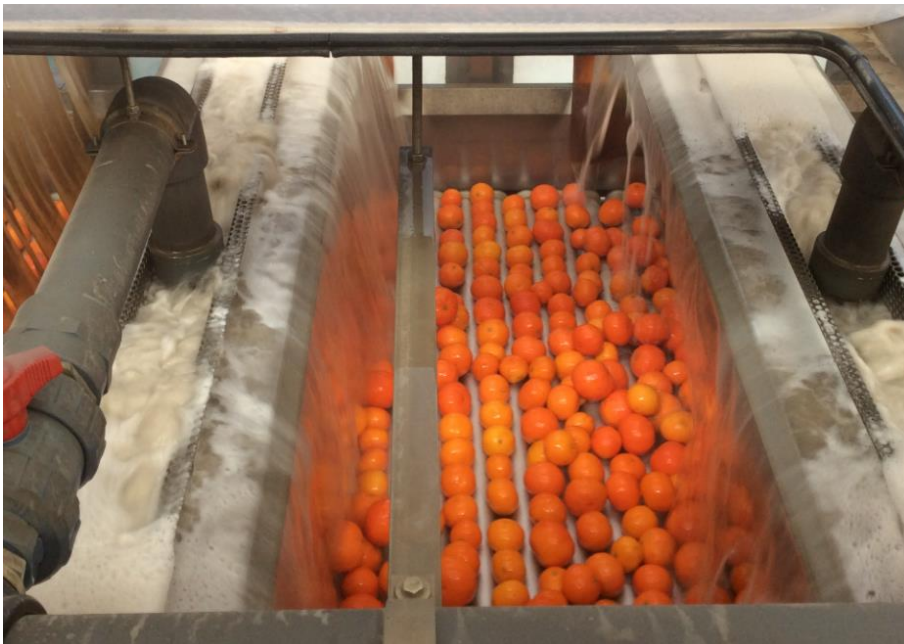
Figura 13. Balsa catarata o drencher on-line.
